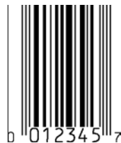
Figure 5.2.2.4-1. UPC-E barcode (encoding 001234000057 by zero-suppression)
