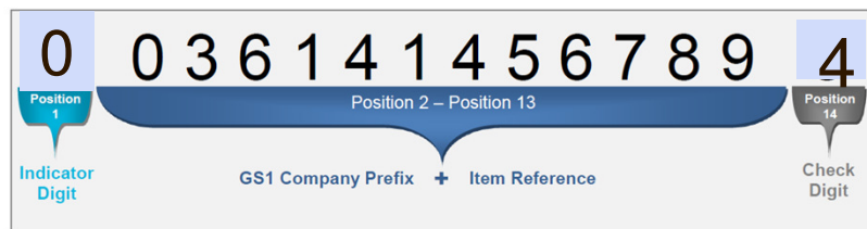
Figure 2. Segments of a GTIN-12 (based on the hypothetical GTIN "361414567894")
