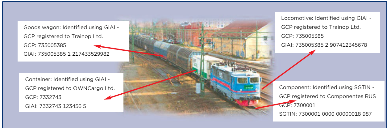
Figure 2-1: The GS1 System has different identification keys for different purposes. The GS1 Company Prefix (GCP) forms a core part of the GS1 Keys to provide a way for GS1 users to uniquely and globally identify different things.
